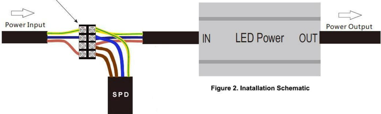
**Figure 2. Inatallation Schematic**
