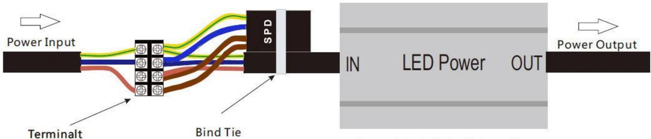
**Figure 1. Inatallation Schematic**
