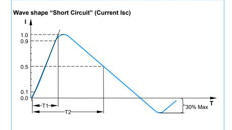
IEC 61000-4-2 Compliant ESD Current Pulse Waveform
